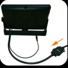
Attach the 26-Pin connector to the monitor
