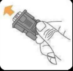
Attach the D-Sub 15-Pin connector to your computer's analog VGA output connector
