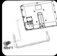
Depending on your application, you can choose to install the included U-Shape bracket onto the monitor
