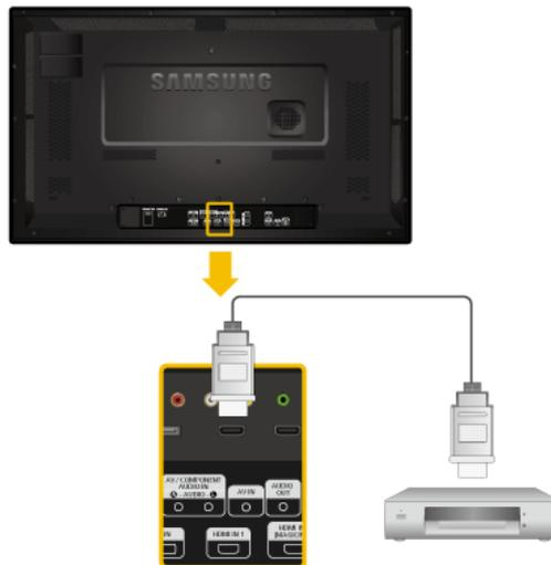
1. Connect an HDMI cable to [HDMI IN 2 (MAGICINFO)] or [HDMI IN 1] on the product and the HDMI output port on a digital device.
