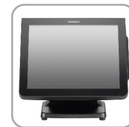
15" Projected Capacitive Touch Spill and Dust Proof
