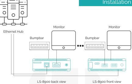
Make sure that all systems are powered off before making or removing any connections to the LS-8900 unit. Follow the steps below in connecting the devices:
