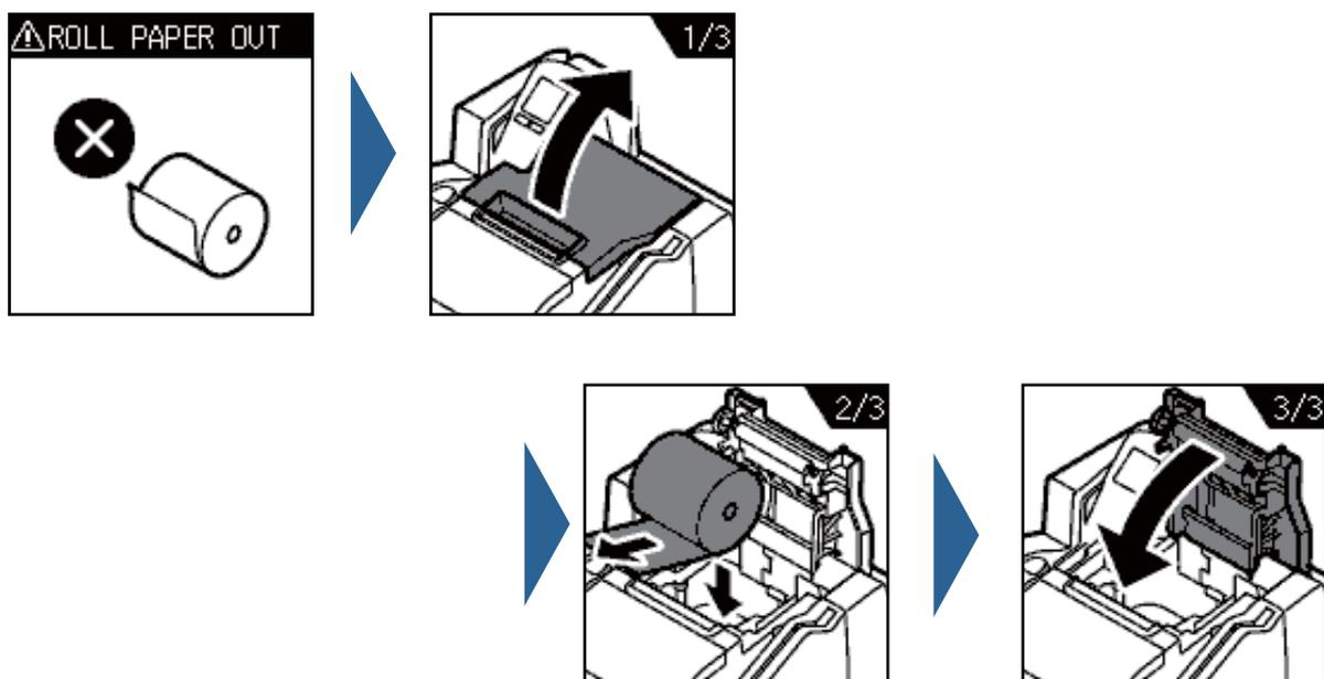
For information on roll paper replacement, refer to [“Loading Roll Paper”](#) on page 40. Replacement can be performed with the same procedure. Do not leave the core of used roll paper in the product.
