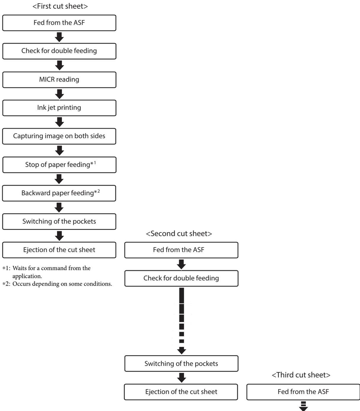
**Without overlap****When back feeding is not necessary with 1-pocket models/2-pocket models**
