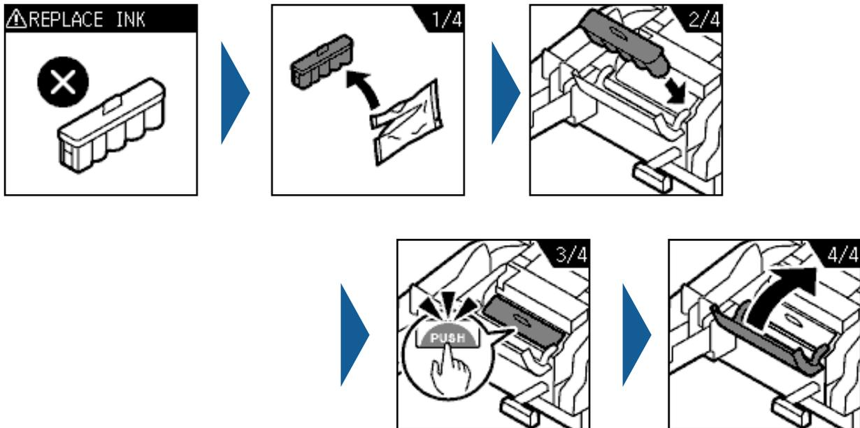
For the replacement procedure, refer to [“Installing the Ink Cartridges”](#) on page 41. Replacement can be performed with the same procedure. Grasping the tab on the top side of the used ink cartridge, pull it out to remove it.
