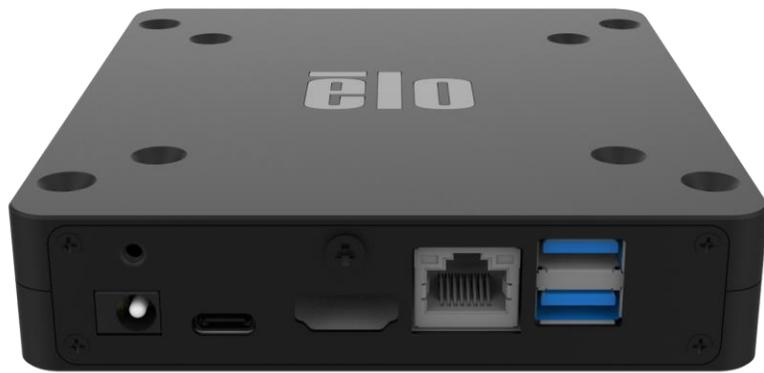
DC In Type C HDMI Ethernet USB 3.0
