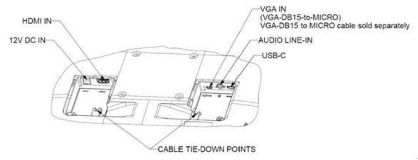
Note: Cable tie-down points can be used to tie down the cables with tie wraps. Simply loop the tie wraps through the cable tie-down points and around the cable to secure cable connections.
