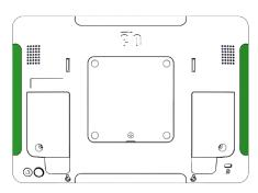
Remove the Edge Connect peripheral covers to expose the mounting interface. Up to two status lights can be installed on a single I-Series display
