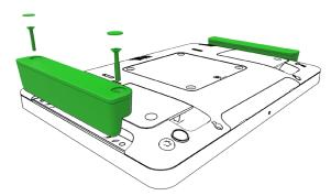
Gently press the status light into the Edge Connect peripheral bay making sure the connector is seated. Then install the included screws and screw covers.
