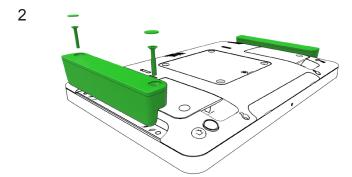
Fasten the status light to the I-Series using the included screws and screw covers.
