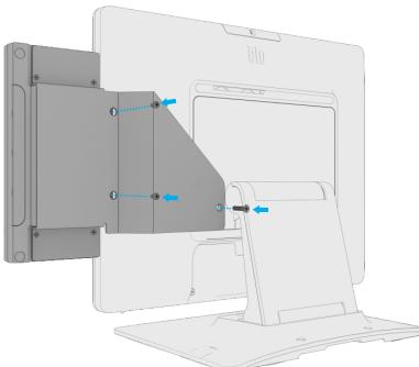
Install the keypad and bracket onto the monitor. Begin by fastening the (2) M3 x 6mm pan head screws provided in the package, followed by the M4 x 18mm flat head screw. Tighten all screws as shown in the illustration.
