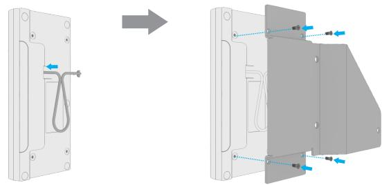
Connect the cable to the keypad. Install the keypad onto the bracket (Select the appropriate bracket compatible with either model 1523L or 1723L). Secure it with the (4) M3 x 7mm flat head screws from the package, as shown.
