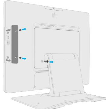
Remove the (2) screws from the peripheral cover and detach the peripheral cover. Then remove the screw from the stand, as shown.
