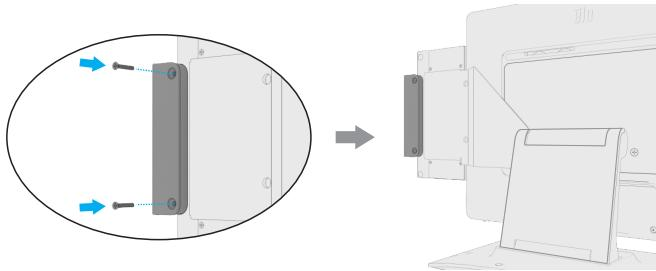
Install the (2) M3x18mm flat head screws from with the kit.
