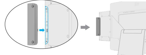
Gently press the MSR into the peripheral bay making sure the connector is mated.
