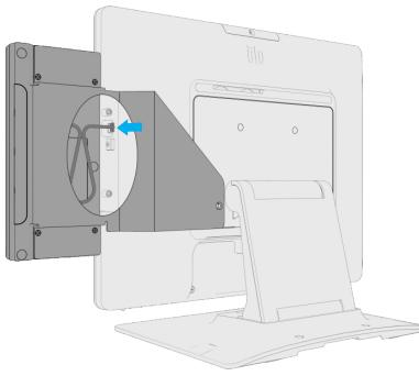
Connect the cable to the monitor.
