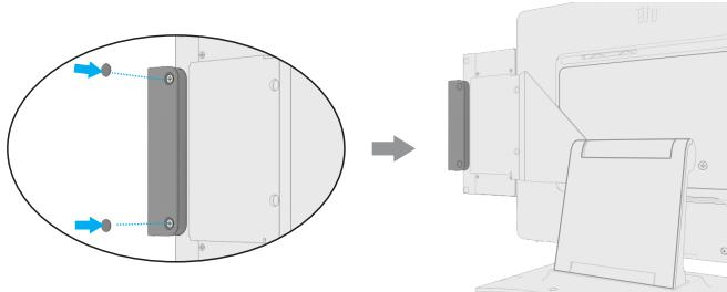
Remove the protective film from the included mylar covers and place the covers over the screws.
