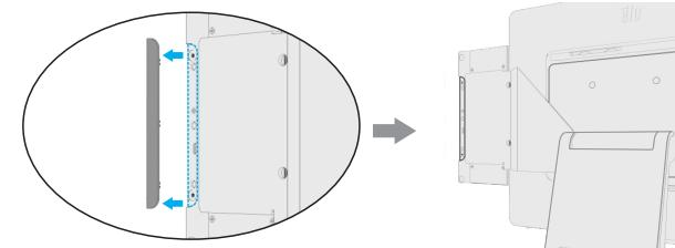
Remove the Edge Cover from the keypad to expose the peripheral bay.
