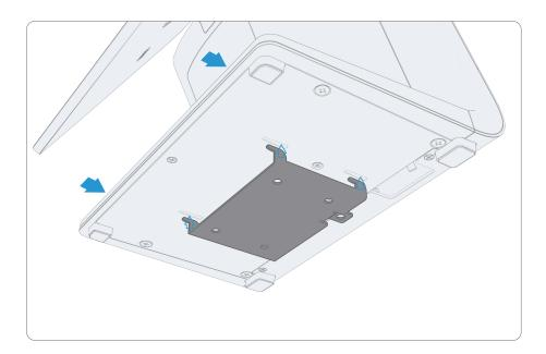
6 Secure the system to the bracket using the M4x8mm screw included in the accessory box.
