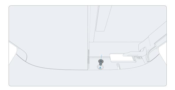
Remove the cable cover door to access the I/O connections.
