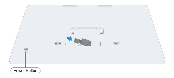
2 Install Windows Slate display on stand, first put the hooks of the bracket into the holes, then lock the bracket using included M4x6mm flat-head srews.
