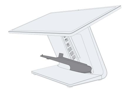
Route the DC power cable through the hole in the bottom of the stand and connect it as shown. Connect other I/O cables as needed (see page 2). Make sure all cables route through the plastic clip at the bottom and re-install cable cover door.
