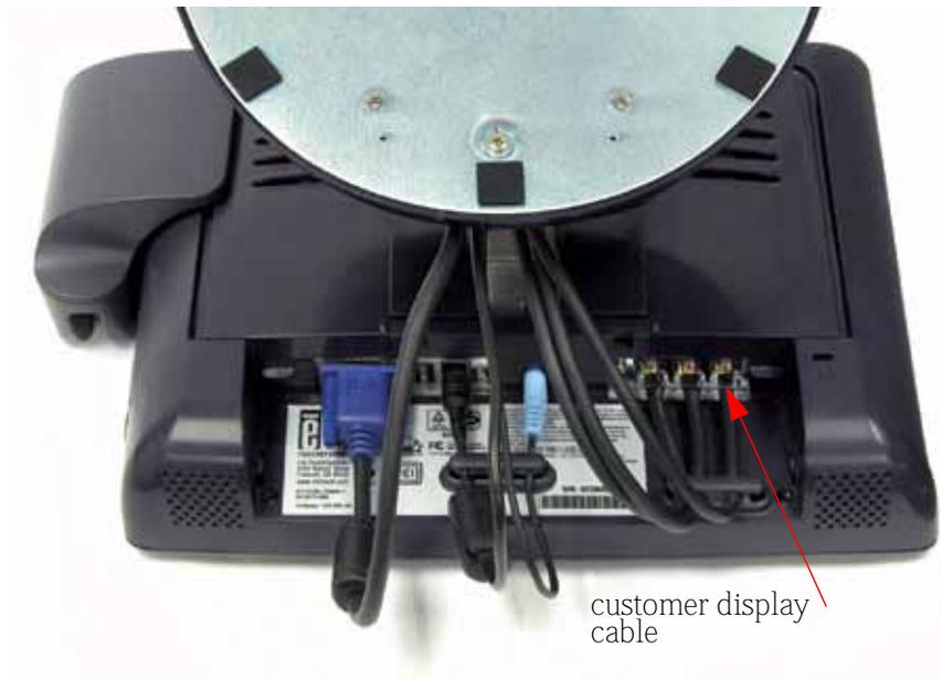
Connect one end of the *customer display cable* to the computer and the other end to the monitor. Secure the cable under the cable management clip.
