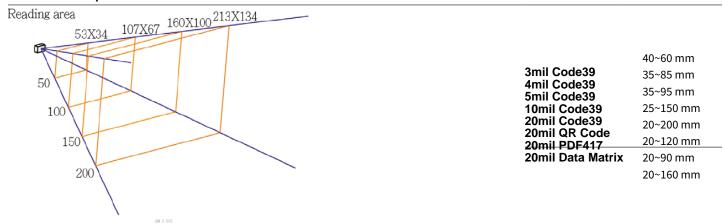
Note: The test is under ambient light 700 ~ 800 Lux.
