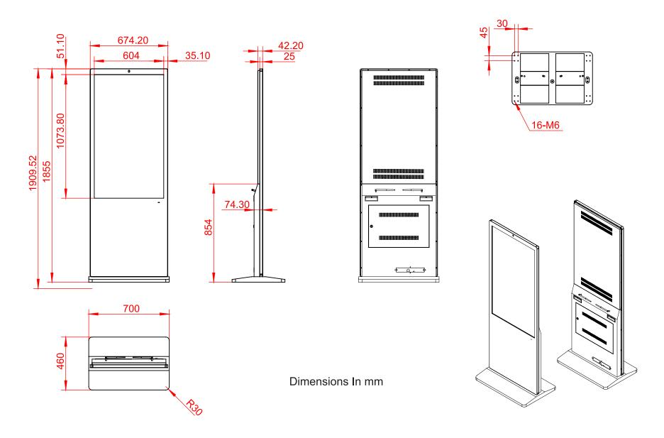
This drawing and it's dimensions are not to be used for fabricating any parts or for any other reasons that are based on these dimensions
