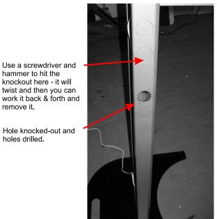
2) Position shelf over the hole and mark 2 locations for drilling using the holes in the shelf arm as a template. Drill 2 holes.
