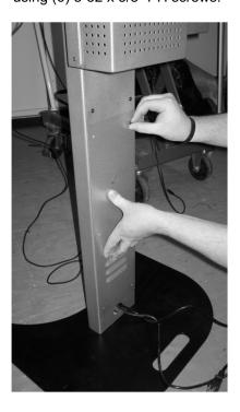
6b) Tidy up the cables using the included cable ties and zip ties. Fish the power cables either out the rear knock-out or through the baseplate.
