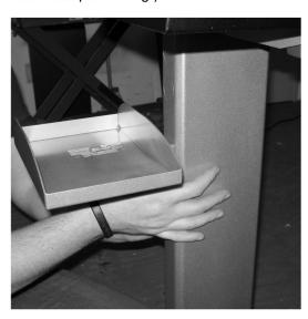
3c) Attach the printer tray using (2) 8-32 x  $\frac{1}{2}$ " PH screws and (2) 8-32 x  $\frac{11}{32}$ " lock nuts as shown.
