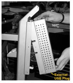
Make sure that the external USB plug cable is attached to the PC before securing the PC housing cover.
