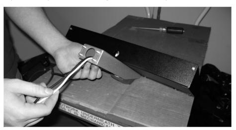
2b) Fish the keyboard cables through the hole in the main support column and fasten the keyboard sub-assembly with (4) 10-32 x 3/8" lock nuts.
