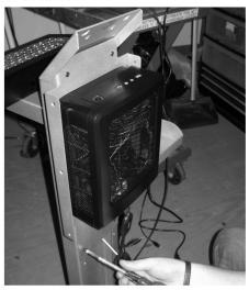
5d) Pull all of the peripheral cables that attach to the PC (LCD, touch, printer, barcode, etc.) through the hole under the PC as shown:
