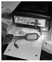
5c) Mount the PC housing subassembly to the top of the main support column. Note the orientation.
