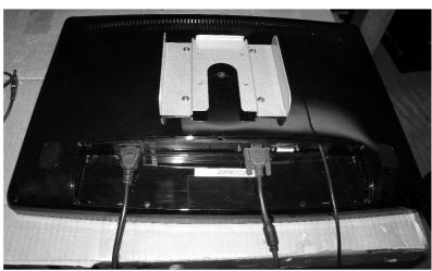
4b) Fish the LCD's video, power, and USB touchscreen cables through the hole at the top of the main support column.
