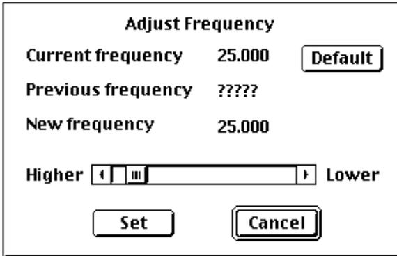
The Adjust Frequency dialog box displays the frequency the touchscreen is currently using and the frequency last used.
