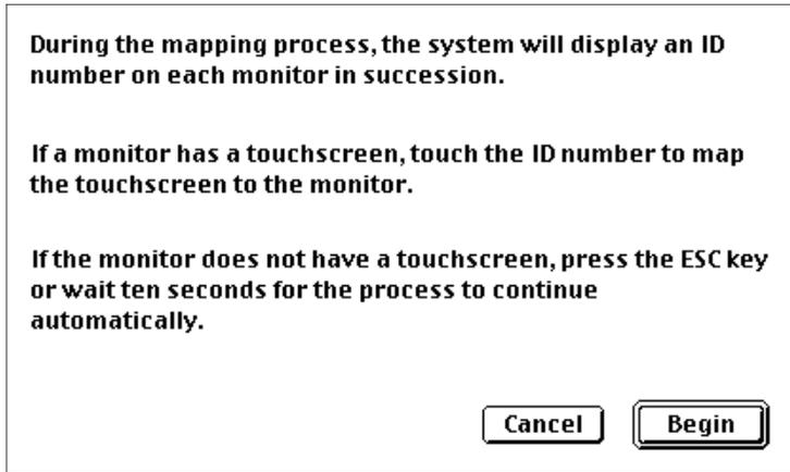
You can select Cancel to exit the mapping procedure. However, if you have modified the monitor configuration of your system, you must map your touchscreens. Failure to do so will result in erratic operation of your touchscreens.
