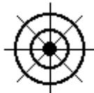
4. Touch the center of the target. Make sure to follow the guidelines described previously in “How to Touch the Screen During a Calibration.” Hold your touch for at least three seconds.
