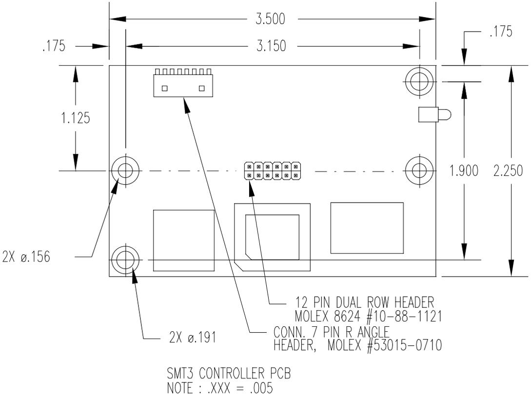
Figure 2. Serial/SMT3 Touchscreen Controller
