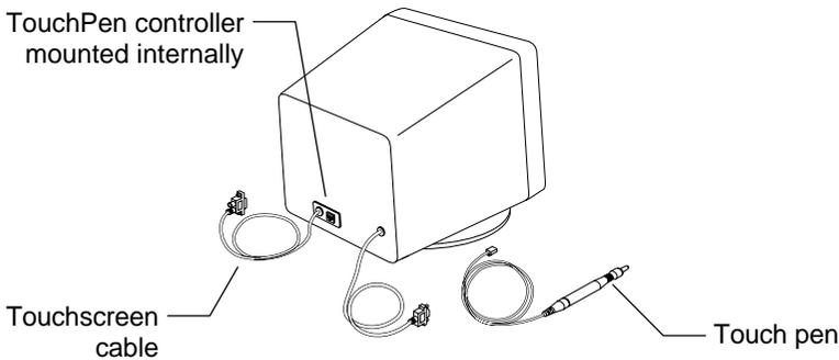
This RS-232 serial controller, which measures a trim 1.35 x 4.8 x 0.3 inches, is designed to easily fit inside flat panel displays and CRTs. The TouchPen controller is always mounted internally.
