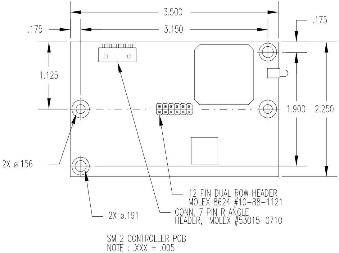
Figure 1. Serial/SMT2 Touchscreen Controller
