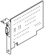
The PC Bus controller is a half-slot, bus card that you install in your system. It has its own serial communication (COM) port, enabling you to use your existing COM ports for other peripherals.
