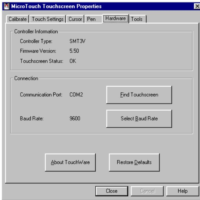
Use the Hardware tab to determine the basic system settings for your touchscreen, verify the touchscreen is communicating properly, select baud rate, and restore system defaults.
