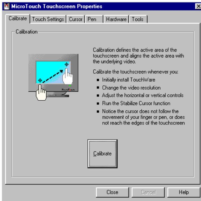
The calibration process aligns the touchscreen with the underlying video. Specifically, calibration defines the dimensions of the active area of the touchscreen and locates the center of the touchscreen. If the screen is improperly calibrated, the active area of the touchscreen may not be aligned or may be unnecessarily small in size.
