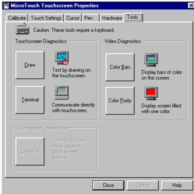
Use the Tools tab to perform basic touchscreen diagnostic tests with the Draw and Terminal programs; video diagnostic tests with Color Bars and Color Purity graphs; and touchscreen linearization if you have a TouchPen controller.
