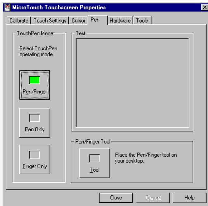
The Pen tab options are available only if your system has a TouchPen controller. TouchPen Mode defines whether the touchscreen recognizes input from both a pen and a finger, from a pen only, or from a finger only. The default mode is Pen/Finger, which means that you can use either your finger or your pen to select options.
