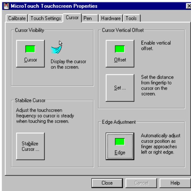
After you calibrate the touchscreen, the cursor should be located directly underneath your finger when you touch the screen. However, you may prefer to offset the cursor slightly above your touch so you can see the cursor and point more easily and precisely to small objects. You can set this and other options for the cursor using this tab.
