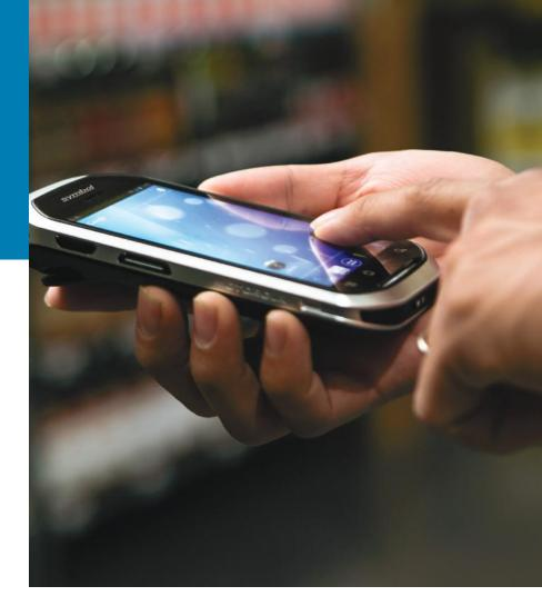
In addition, you can process payments with Chip and PIN-based debit and credit cards by pairing the MC40 with Zebra's Bluetooth PD40 Payment Device.
