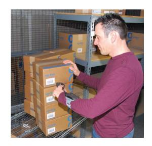
The Socket Bluetooth® Cordless Ring Scanner Series 9 is a wearable, hands-free barcode scanning solution that improves productivity in processes that involve repetitive scanning and package or parts handling tasks.
