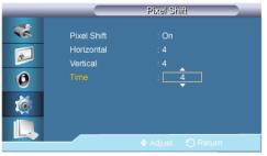
Set the time interval for performing the horizontal or vertical movement, respectively.
