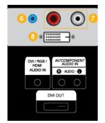
6 DVI / RGB / HDMI AUDIO IN (PC/DVI Audio Connection Terminal (Input))
