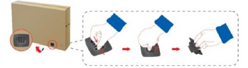
Remove the lock from the package box, as shown in the figure above.
