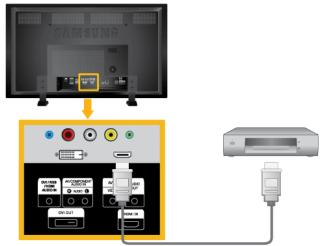
1. Connect input devices such as a Blu-Ray/DVD player to the HDMI IN terminal of the LCD Display using an HDMI cable.
