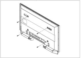
2. Insert the screw B into the plastic hanger.
