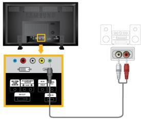
1. Connect a set of audio cables between the AUX L, R jacks on the AUDIO SYSTEM and AUDIO OUT on LCD Display.
