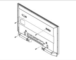
4. Remove safety pin (3) and insert the 4 product holders into the corresponding bracket holes (1). Then place the product(2) so that it is firmly fixed to the bracket. Make sure to re-insert and tighten the safety pin (3) to securely hold the product to the bracket.
