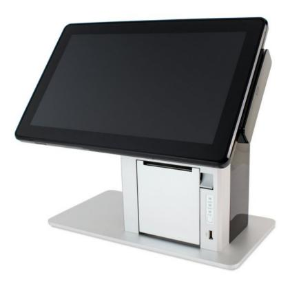
Sleek, stylish, with a compact design the TP5 is perfect for even the most confined POS locations. The TP5 features a TruFlat projected capacitive touchscreen, quad-core CPU, built in printer.
