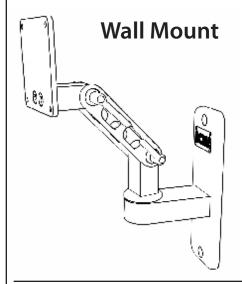
Locate the stud in the wall you are mounting to and mark the top hole. Drill 11/64 pilot hole and insert the provided #14 wood screw, tightening slightly. Using a level, mark the lower hole and drill pilot hole, insert the last #14 screw and, with the unit level, tighten both screws.
