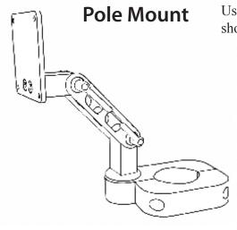
Using the 1/4" hex key, separate the two halves of your pole mount as shown, place around pole at the desired height and reassemble.
