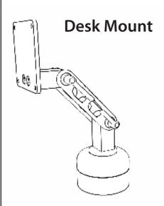
Drill a 3/8 hole through the horizontal surface you intend to mount to and push the 3/8 stud on the desk mount through the hole. Slip the large mounting washer over the stud from underneath, add the 3/8 split-washer, and secure in place with the 3/8 nylock.
