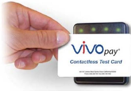
This tests the antenna's ability to read the RFID test card. If unsuccessful, there will be no reaction from the reader. If you use a test card and the ViVOPay reader is attached to the ViVOPay Kiosk II Controller, a dummy transaction can be tested. The transaction will not be authorized and will come back with a response, but will at least test for end-to-end connectivity.
