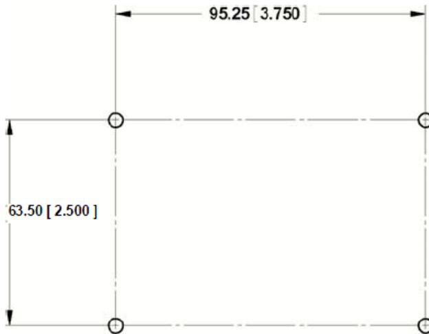
3. Drill the four 4.4 mm (0.173 inch) mounting holes using a number 17 drill bit.
