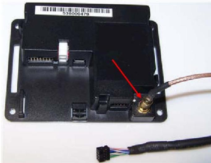
2. Attach the other end of the cable (220-2457-00) from the antenna to the ViVOpay Kiosk II Controller.
