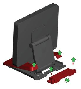
Remove stand cover using coin or other tool. Remove the two screws holding the rear portion of the stand cover on and remove the cover.
