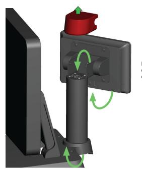
Remove pole hinge cover and route cables through pole and connect to computer. Reinstall pole cover.
