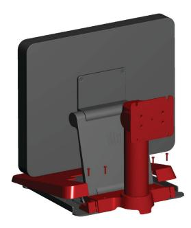
Place pole mount on back of stand and align the screw holes. Install the (4) M4x14 screws to fasten the stand and then replace the cover.
