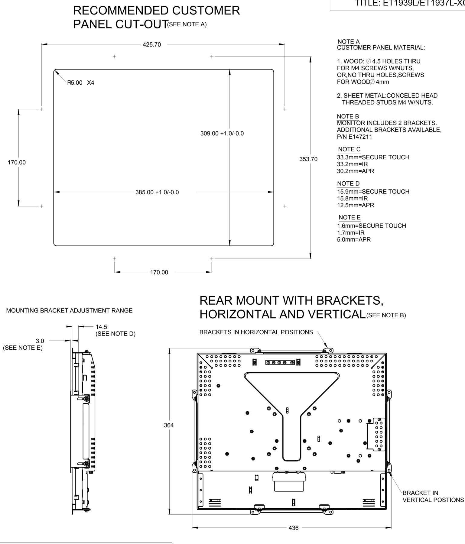
DIMENSIONS ARE IN MILLIMETERS
