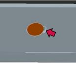
Carefully insert a small flathead screwdriver under the open edge of the cover and peel the cover up.
