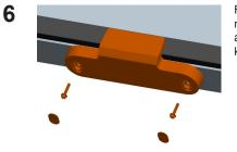
Fasten the reader module to the monitor using the two M3 screws and screw covers supplied in the kit.
