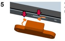
Connect the RFID reader power cable to the connecter in the center peripheral hole.
