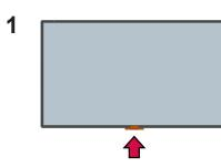
The RFID Reader can be attached to any of the 4 sides of the touchmonitor. Elo suggests the bottom side for ease of use.
