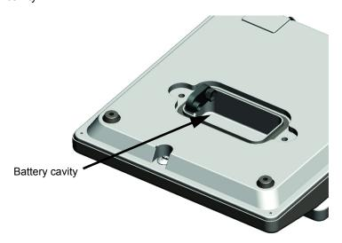
3. Install the 9V alkaline battery
