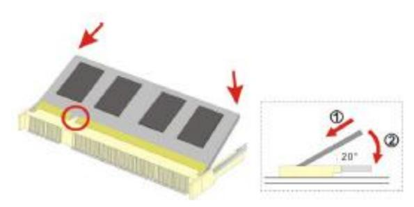
Figure 2.4: Installation of Memory Module
