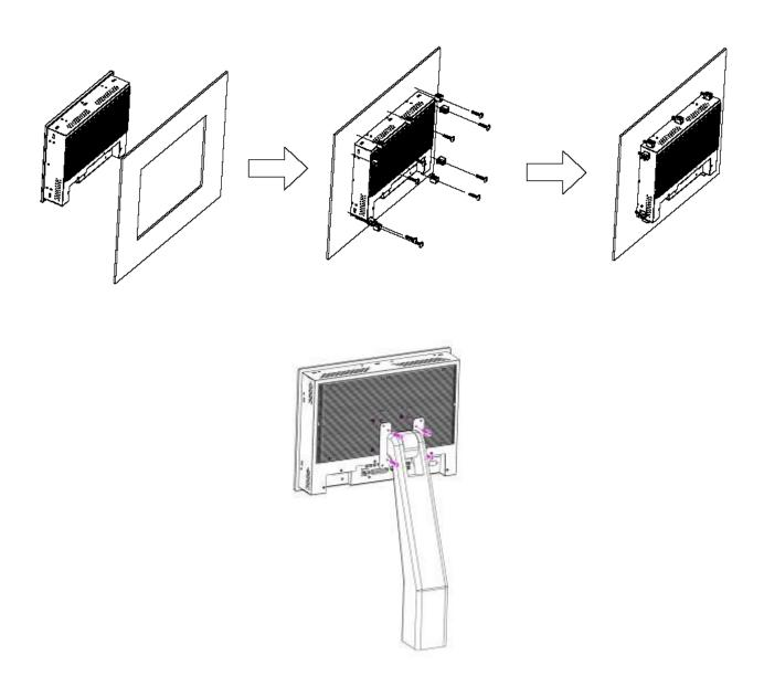
Figure 1.9 Panel mounting and VESA mounting of the AHM-6xx7A
